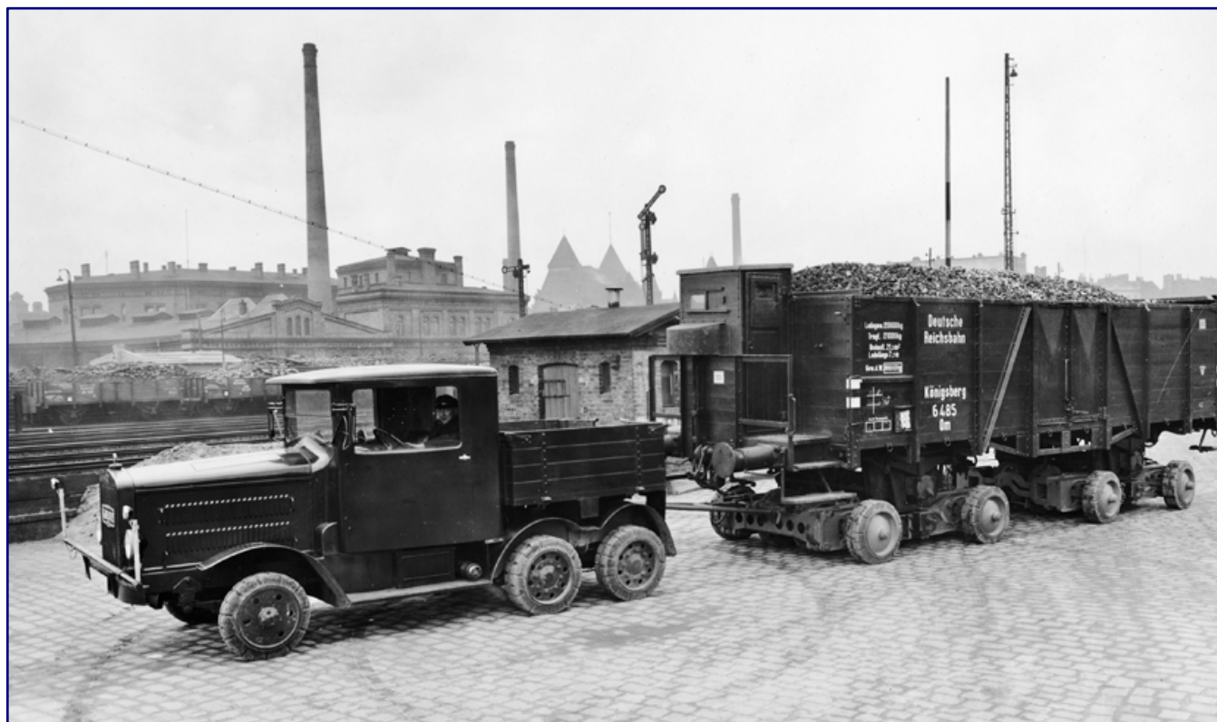
On 27 April 1933 the Reichsbahn in Berlin-Anhalter Gbf carried out test runs with the first Culemeyer team. The tractor is a Kaelble Z 6 R with 100 HP power. Only three tractors of this type were delivered to the Reichsbahn. Photo: RVM, Archiv Eisenbahnstiftung
