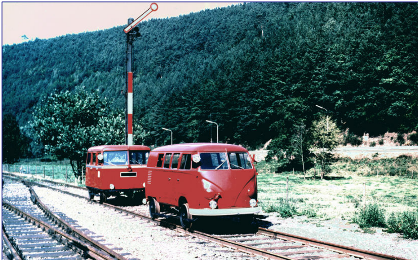
To save development costs, the Klv 20 was derived from a road vehicle. However, it was by no means the only railway master hand car in the service of the DB. On 17th September 1978 two types of construction were presented to the public in Elmstein, among them Klv 20-5011. Photo: Manfred Britz
