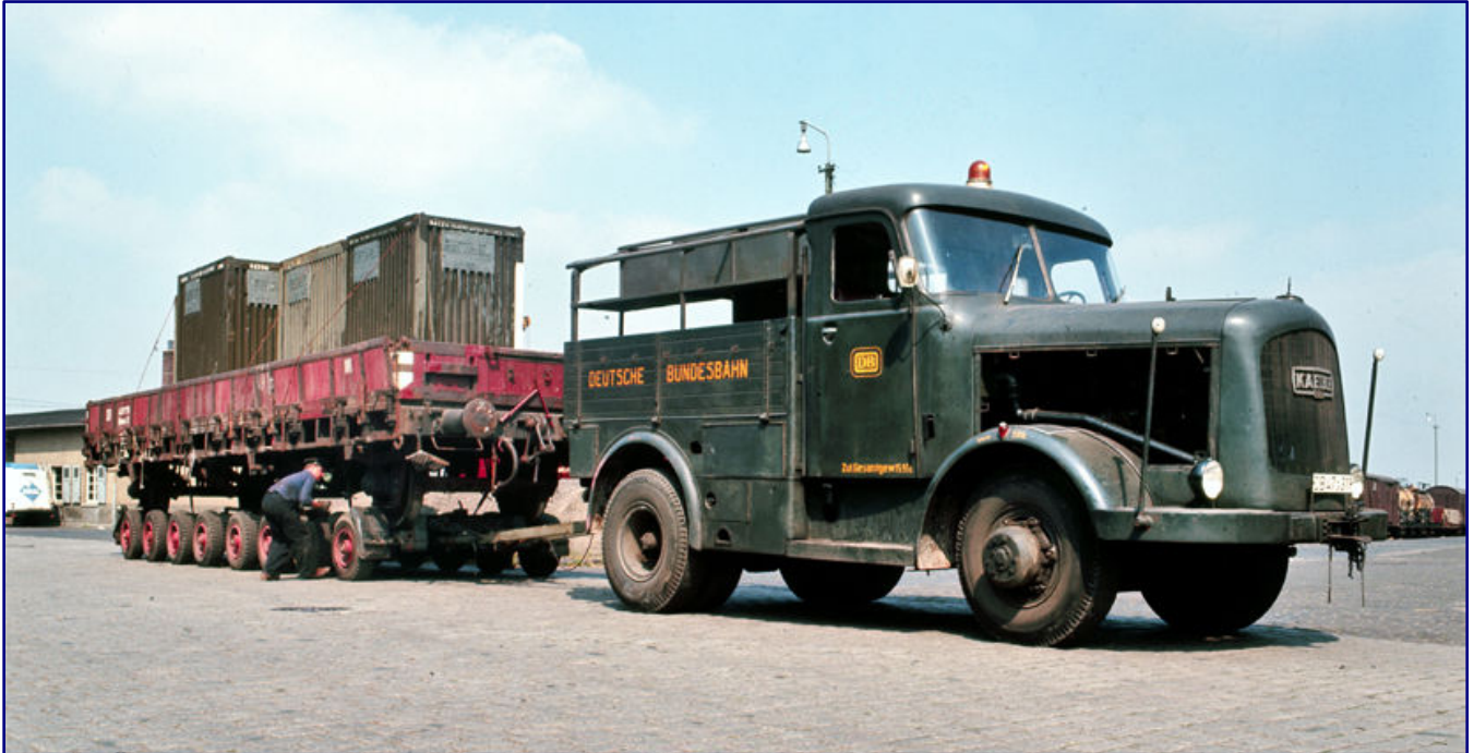
In 1964 a Culemeyer transport with the Kaelble tractor KV 631 ZR 58 (DB 47-311) stands in front of Frankfurt's main freight station, where today the exhibition centre is located on Osloer Straße. The driver checks the correct position of the Rmms 33 on the attached LR 40 road scooter before the transport can begin. Photo: Reinhold Palm, Archiv Eisenbahnstiftung
