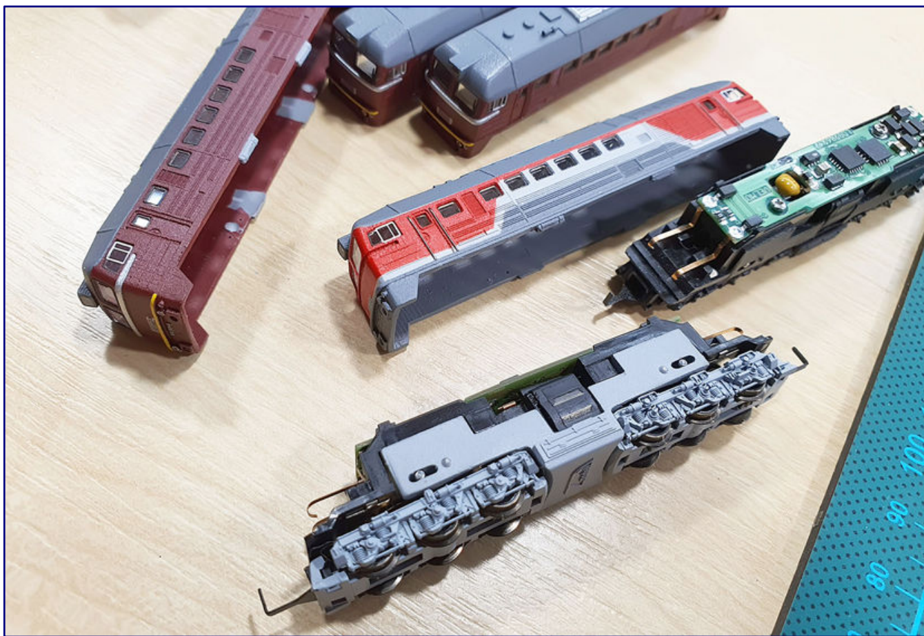
Chassis and bogies are based on parts from Märklin: The bogies were donated by the class 243 electric locomotive (from 1992: 143) and was shortened a little in the plastic parts. The cast block between the wheels had to be milled off and received a cover. The bogies are from the Ludmilla.
