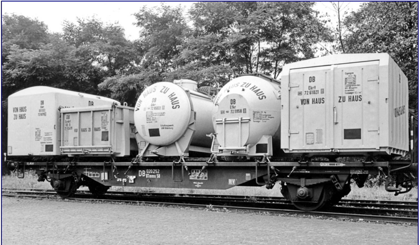
The five-passenger BTmms 58 carrying wagon marks the final stage of development for door-to-door traffic and represents the wagons of similar design built up to 1971. It was built in series from 1960. The open (2nd from left) and closed containers (far right) were the two original types, whereby the open already belongs to a further developed design (model for Märklin). Deep-freeze containers (far left) and those for liquids (centre) as well as moisture-sensitive fine bulk goods (to the right) are the first special types. Photo: Bustorff, Eisenbahnstiftung
