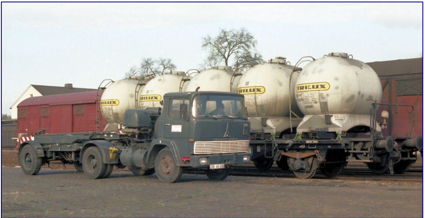
The basic idea of Pa container traffic could probably not be illustrated more appropriately in one picture. The central containers of Trilux, the light source manufacturer from Sauerland, have arrived by rail in Neheim-Hüsten. There they will now change to the Ackermann trucks at the loading dock
