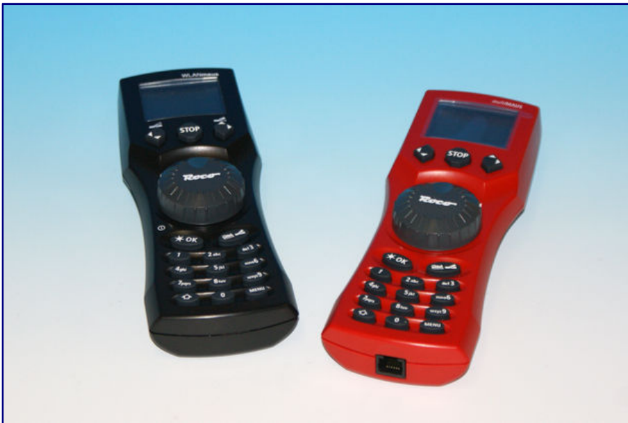
The multi-mouse from Roco (right), which is also used in Z gauge, is both a handset control and a small central unit. It can also switch points or mechanical signals. Its modern successor is the WLAN mouse (left) from the same manufacturer.
